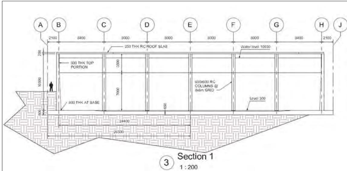
Figure 5. Detail showing sub-surface depth (~ 3.2m) to which the proposed construction will extend
