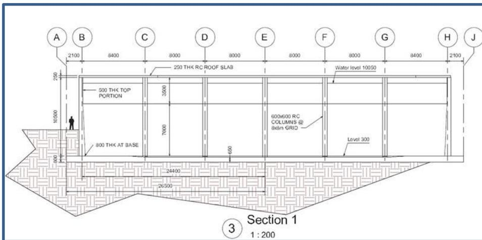
Figure 4. Detail showing sub-surface depth (~3.2 m) to which the proposed construction will extend (from SVA International).
