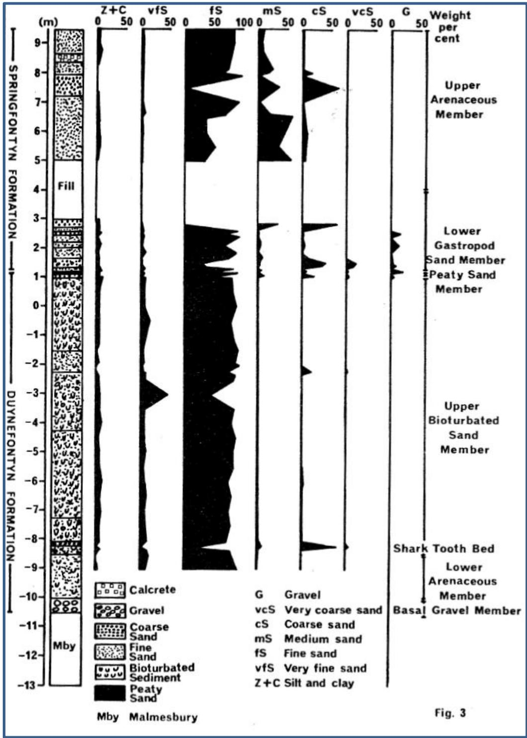
Figure 7. Stratigraphy and lithology recorded in the excavations for the Koeberg Nuclear Power Station reactors (Rogers, 1979), fig 3. Duynefontyn Formation = Varswater Formation.
